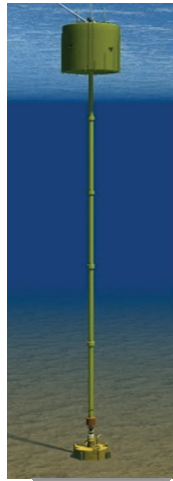
Self-Standing Riser (SSR)
