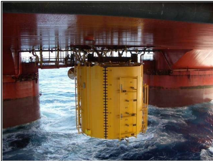
Figure 7 – Self Standing Riser Buoyancy Device Run in the Gulf of Mexico
